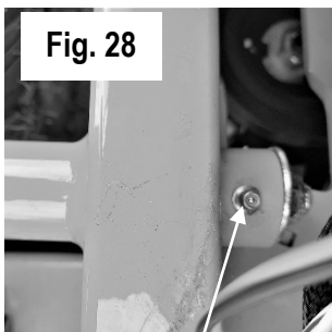
Right Actuator Bar Grease Fitting
